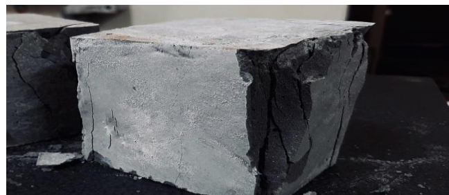
Figure 5: Crushed cement specimen.
