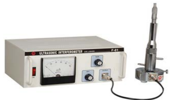
Fig. 5: Experimental Setup: Ultrasonic Interferometer.
