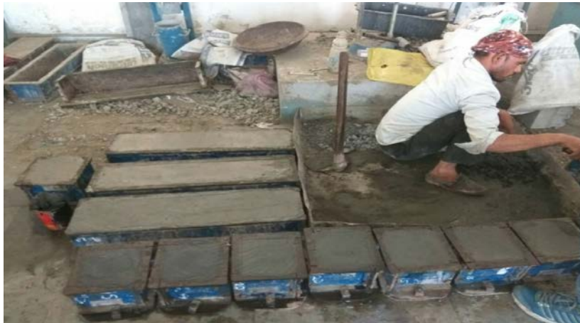
Figure 3: Casting of Concrete Cubes and Beams.
