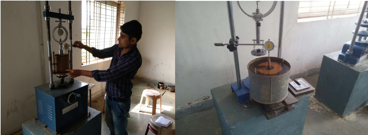
Figure 1: Soaked CBR sample & Swelling test apparatus for 96 Hours.
