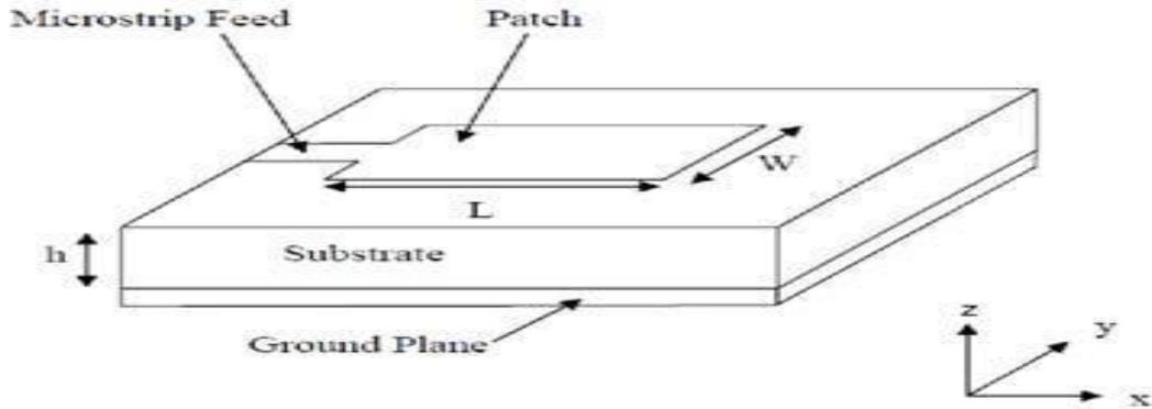
Figure 1: Microstrip Patch Antenna.
