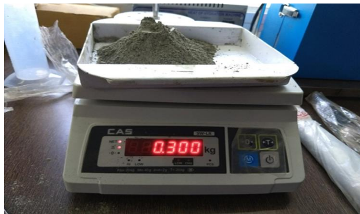
Figure 2: Grade 53 Ordinary Portland cement Sample.
