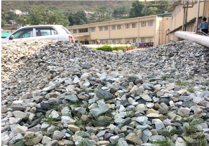
Figure 5: Coarse aggregates of 10 mm size Sample.
