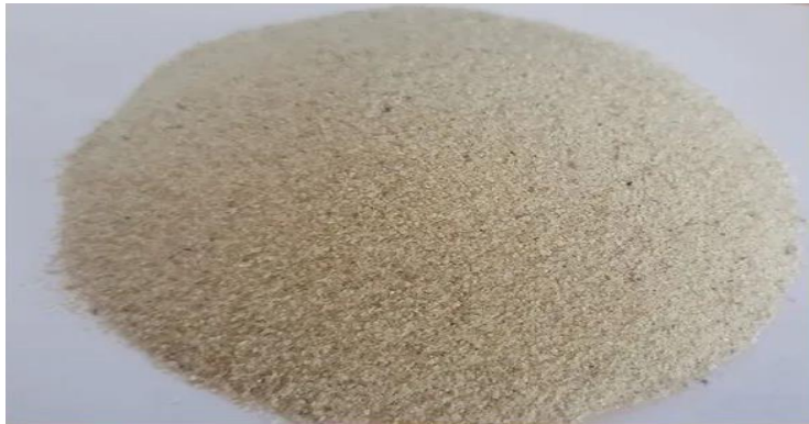
Figure 3: Foundry Sand Sample.
