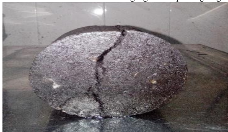
Figure 2: Loading and Failure Pattern Of Indirect Tensile Strength Test.
