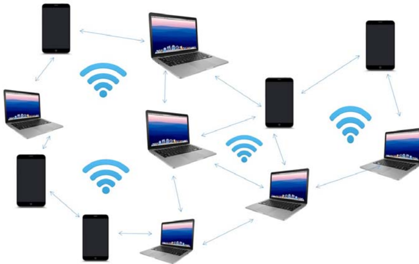
Figure 1: Example of mobile ad hoc network (MANET) structure [2].
