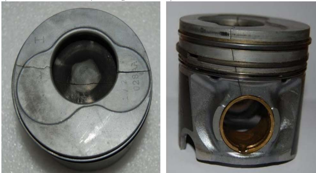
Fig.1.2. A crack on the piston pin: a) cracked piston head; b) cracked piston skirt.
