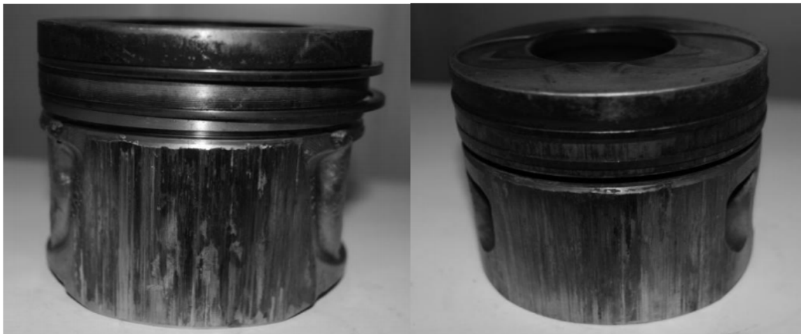
Fig.1.1. A piston skirt seizure.
