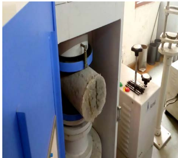
Figure 1: Split Tensile Strength Test.
