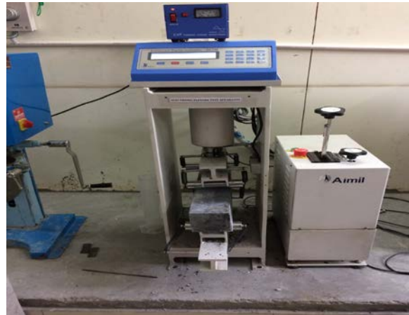
Figure 2: Flexure Strength Test.
