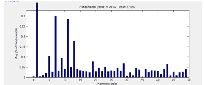
Fig. 11 Harmonics spectrum with Fuzzy controller
