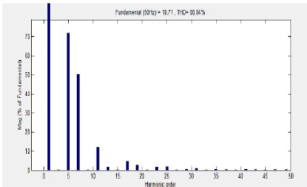
Fig. 9 Harmonics spectrum without controller
