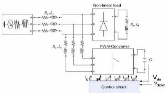
Fig. 2 Active filter controlling system.
