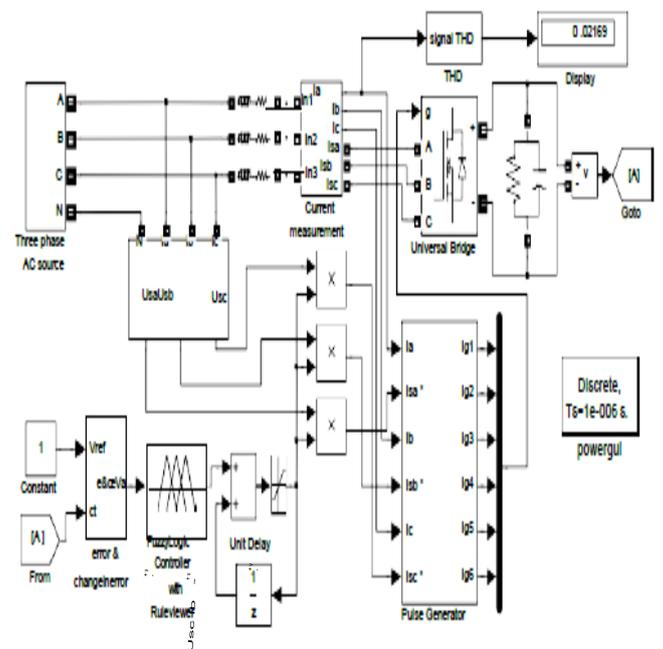
Fig. 7 Simulated power circuit for Fuzzy controlled improved power quality converter
