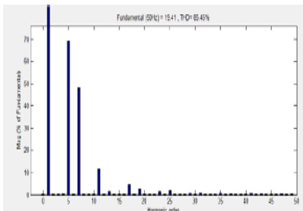
Fig. 10 Harmonics spectrum with PI controller
