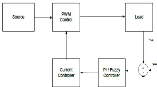
Fig. 4 Block Diagram of PI/Fuzzy controlled improved power quality converter
