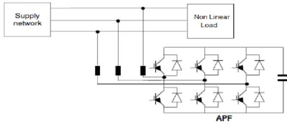
Fig. 1 Active power filter connected with transmission line
