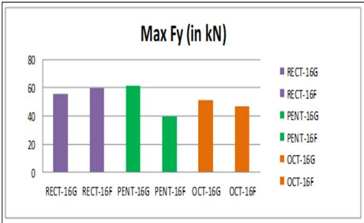
**Graph 2:** Maximum Shear in Y directions for 16storey models.
