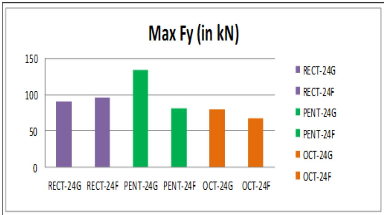
**Graph 5:** Maximum Shear in Y directions for 24storey models.
