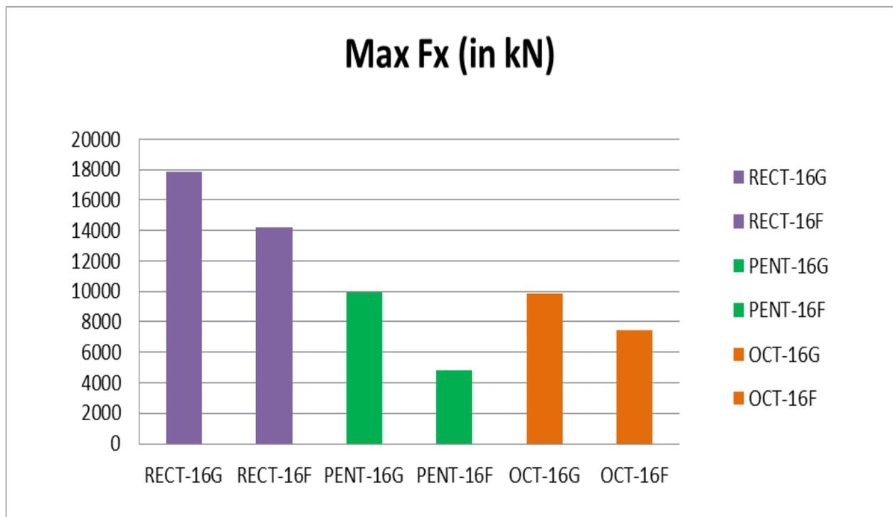
**Graph 1:** Maximum Shear in X directions for 16storey models.
