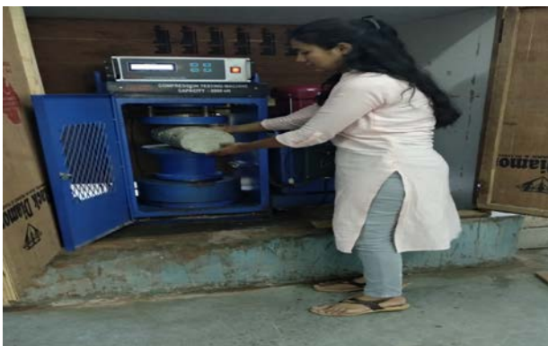
Figure 4. Splitting tensile setup
