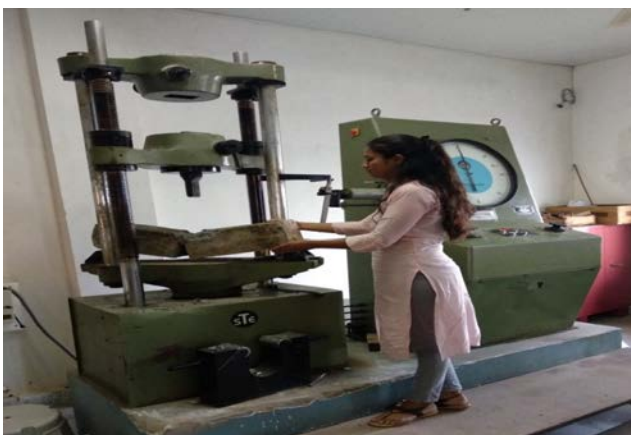
Figure 3. Flexural test setup
