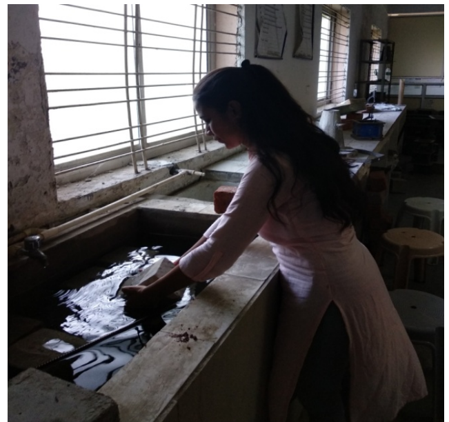
Figure 1. Curing of concrete
