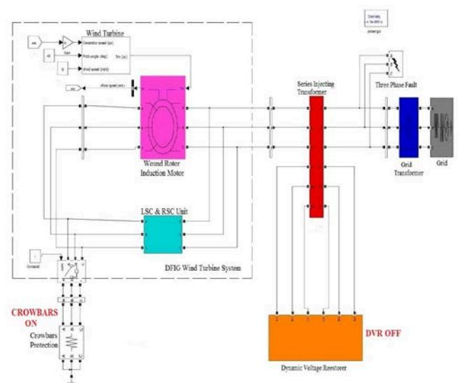
**Fig. 4.2** Simulation Model with Crowbars ON
