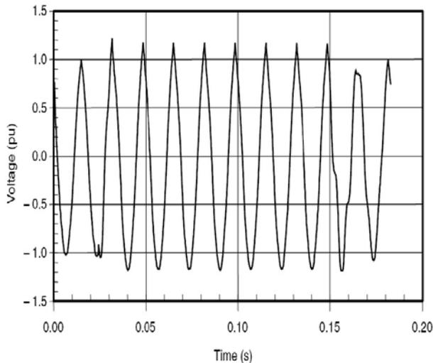
**Fig. 1.2** Voltage Swell Waveform
