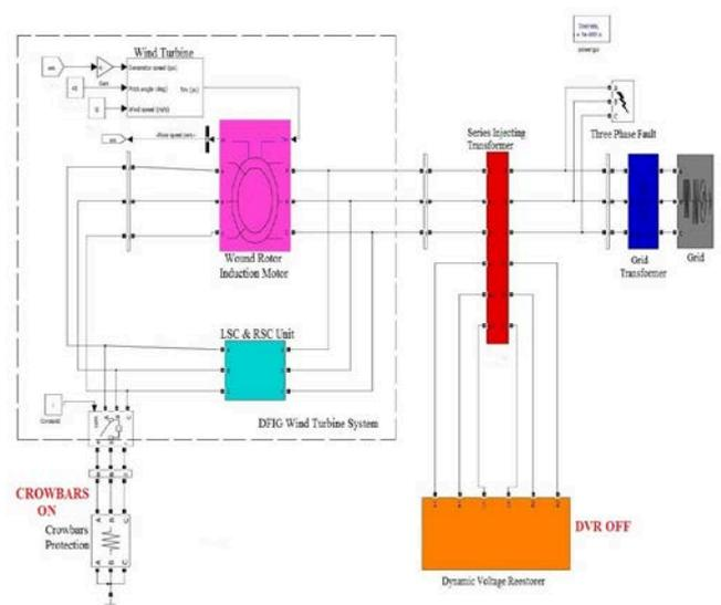
**Fig. 4.2** Simulation Model with Crowbars ON
