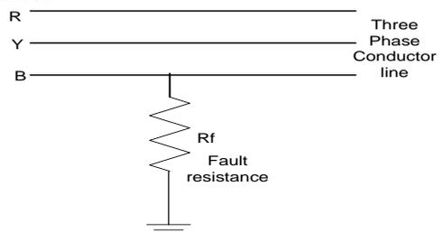
(a) Single Phase to Ground Fault (L-G)
