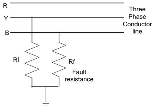
(b) Two Phase to Ground Fault (L-L-G)
