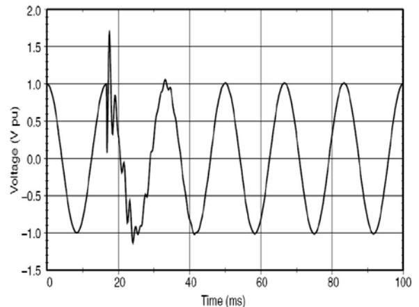
**Fig. 1.4** Oscillatory Transient Waveform
