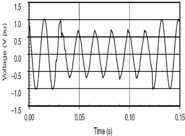
**Fig. 1.1** Voltage Sag Waveform
