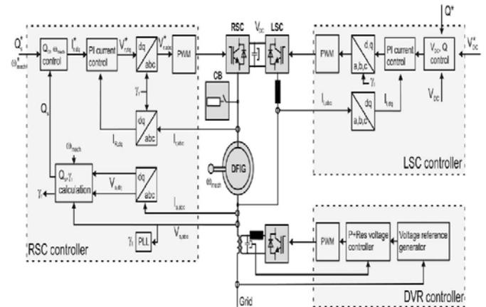
Fig. 3.2 Control System of DFIG & DVR
