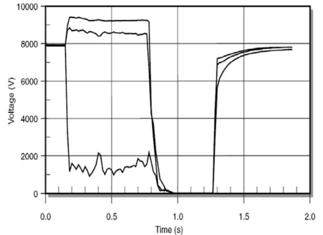
**Fig. 1.3** Voltage Interruption Waveform
