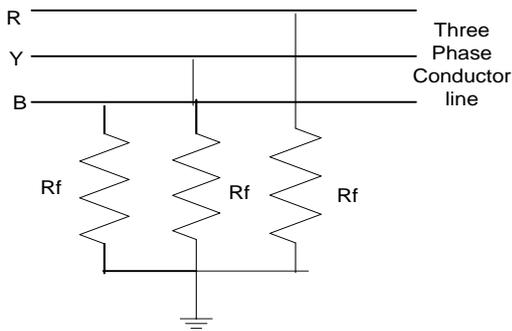
(c) Three Phase to Ground Fault (L-L-L-G)
