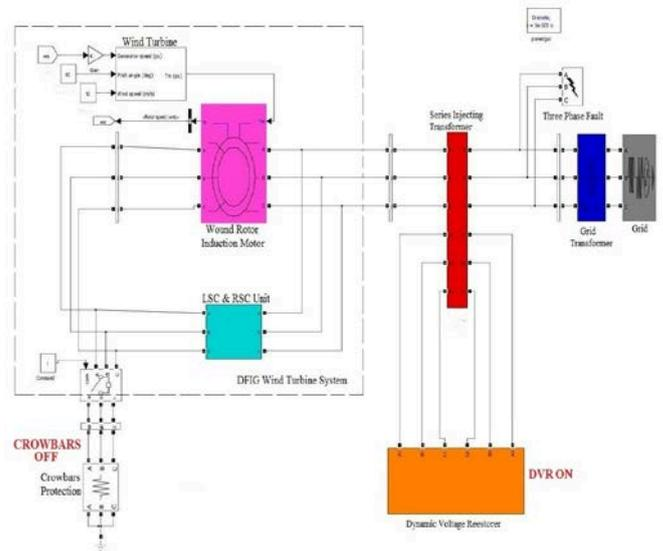
Fig. 4.5 Simulation Model with DVR ON
