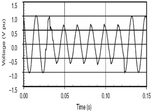
**Fig. 1.1** Voltage Sag Waveform
