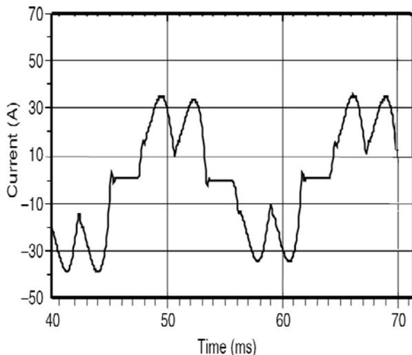
**Fig. 1.5** Waveform with Current Harmonics
