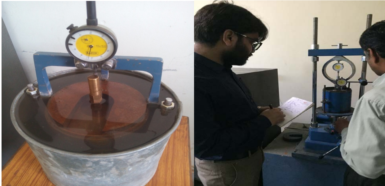
Figure 7: Working process of CBR lab test
