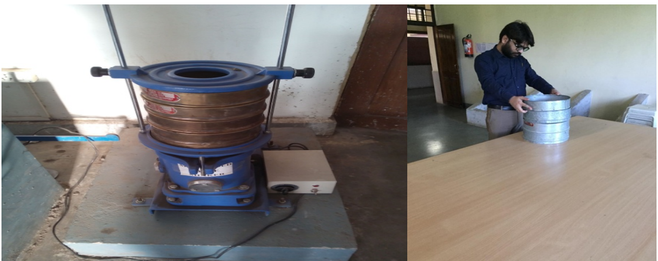
Figure 3: Sieve Analysis Apparatus (Motorised Sieve Shaker)
