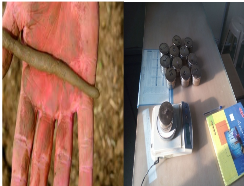
Figure 5: Liquid Limit, Plastic Limit Apparatus
