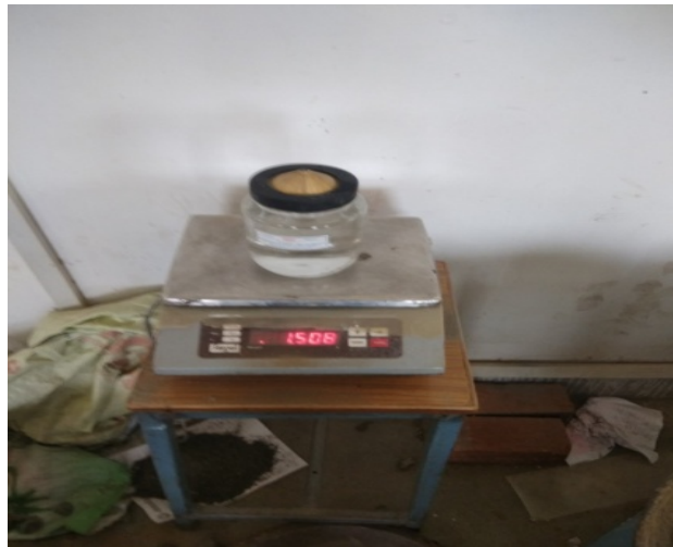
Figure 4: Specific Gravity test Apparatus (pycnometer)
