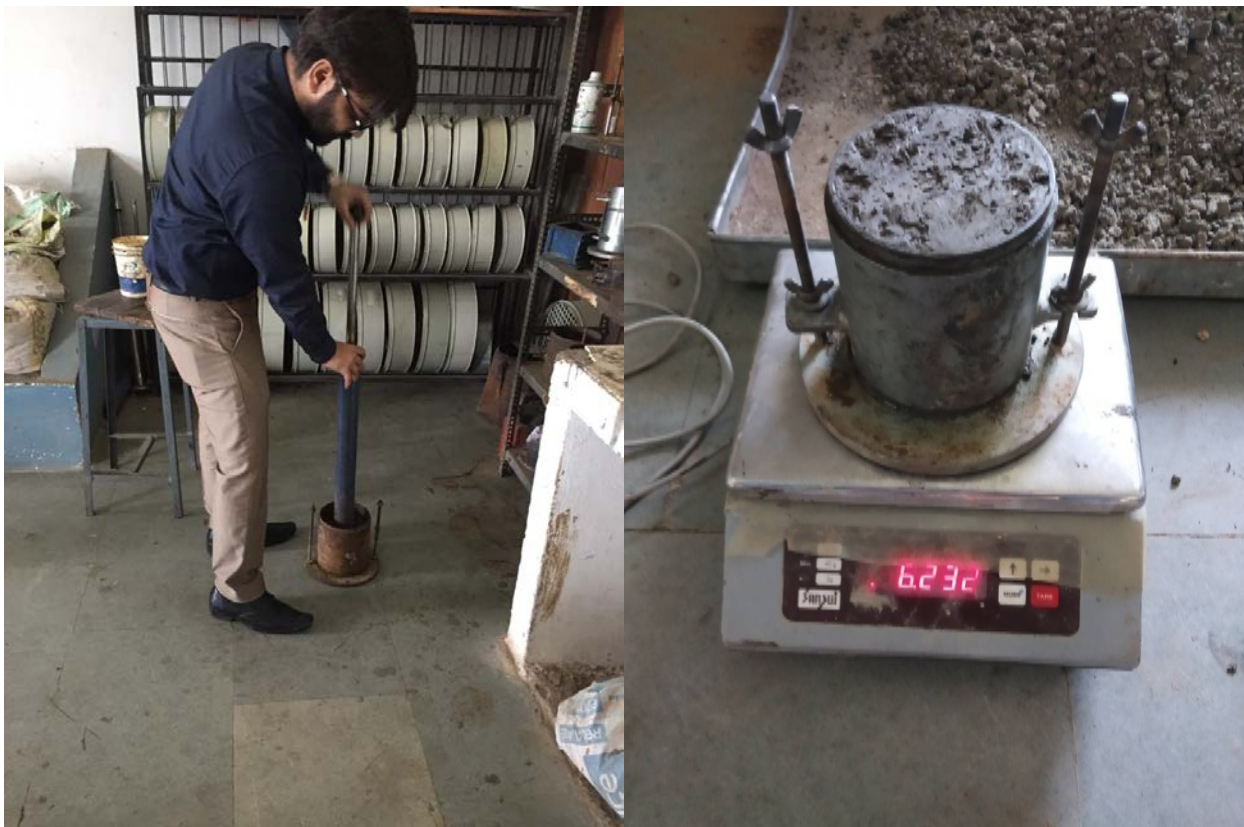
Figure 6: Rammer Apparatus and Sample Prepare for Compaction Test
