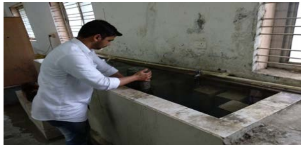
Fig 2. Curing of concrete
