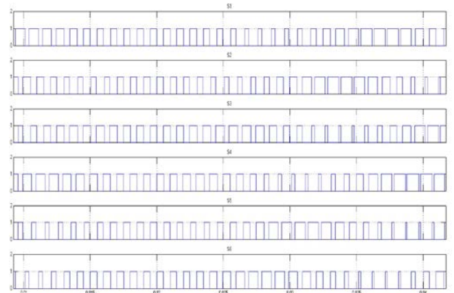
Fig 10: Gate firing Pulses for Three Phase Inverter.
