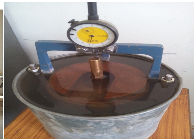
Image 6: Test Samples for Soaked and unsoaked CBR
