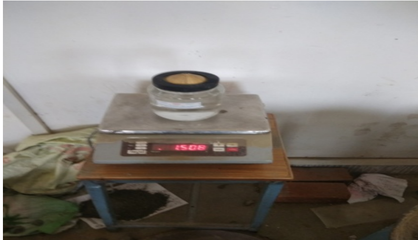
Image 3: Specific Gravity test Apparatus (pycnometer)
