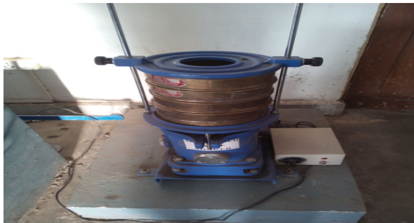
Image 2: Sieve Analysis Apparatus (Motorised Sieve Shaker)
