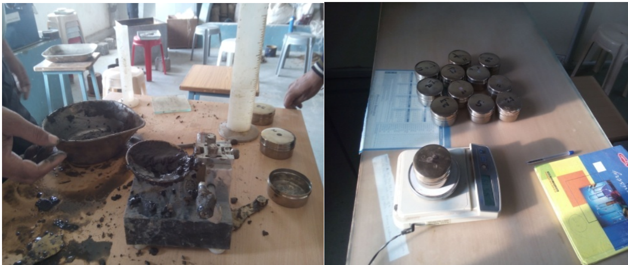
Image 4 : Liquid Limit, Plastic Limit Apparatus
