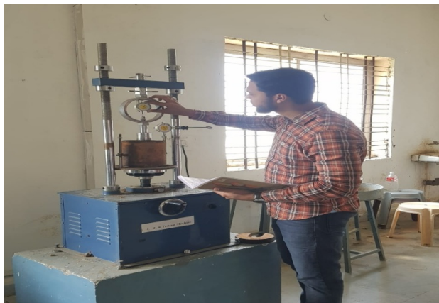
Image 6: Test Samples for Soaked and unsoaked CBR
