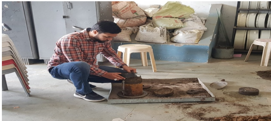
Image 5: Rammer Apparatus and Sample Prepare for Compaction Test
