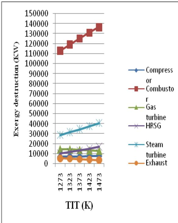
Figure 11: Effect of TIT on Exergy destruction rate in different components of combined cycle at  $R_p = 12.2$ .
