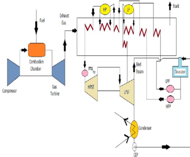
Figure 1: Schematic diagram of combined cycle power plant.
