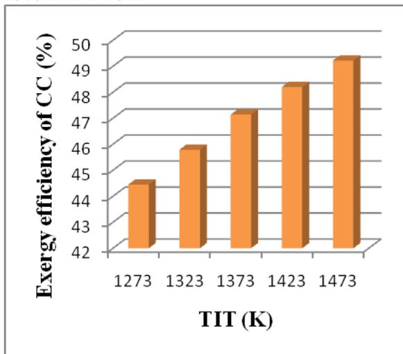
Figure 9: Effect of TIT on Exergy efficiency of combined cycle at  $R_p = 12.2$ .
