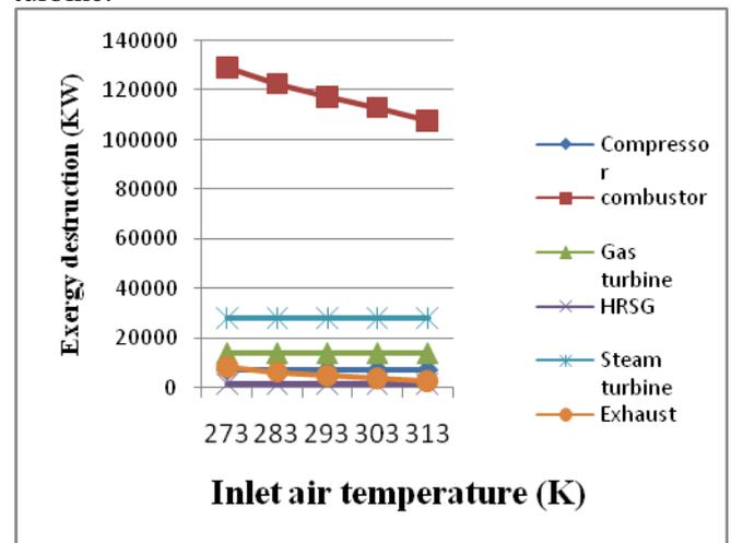
Figure 8: Effect of inlet air temperature on Exergy destruction rate of different components of combined cycle at TIT 1005<sup>0</sup>C and R<sub>p</sub> =12.2.
