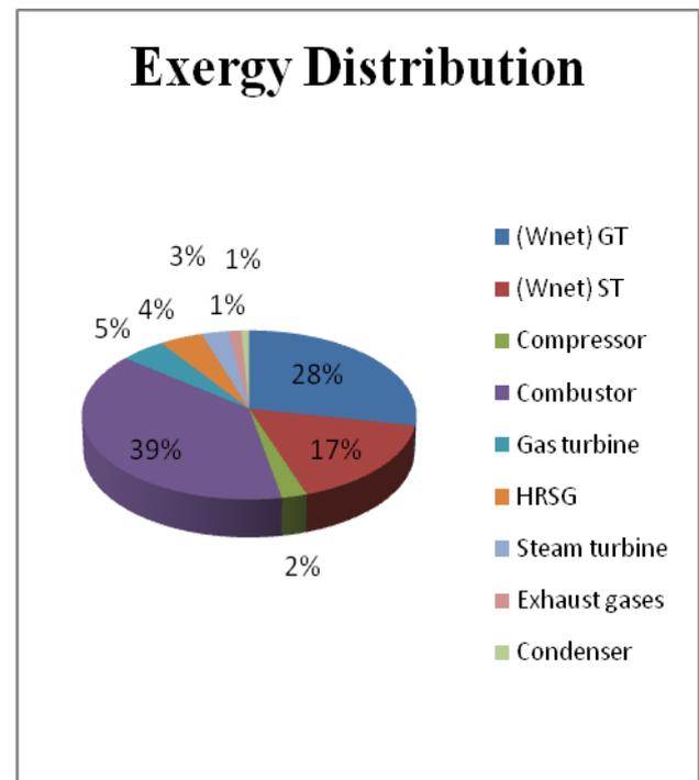
Figure 5: Exergy balance for the combined cycle plant.
