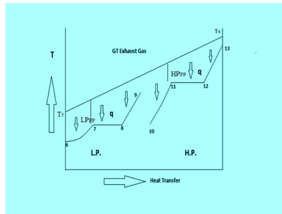
Figure 3: temperatures – heat transfer diagram of HRSG.
