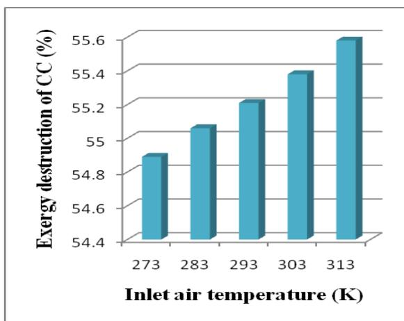
Figure 7: Effect of inlet air temperature on Exergy destruction of combined cycle.
