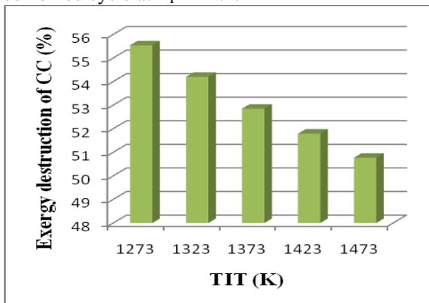
Figure 10: Effect of TIT on Exergy destruction of combined cycle at  $R_p = 12.2$
