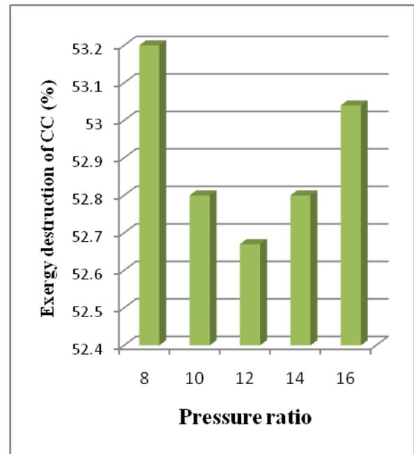
Figure 13: Effect of pressure ratio on Exergy destruction of combined cycle.
