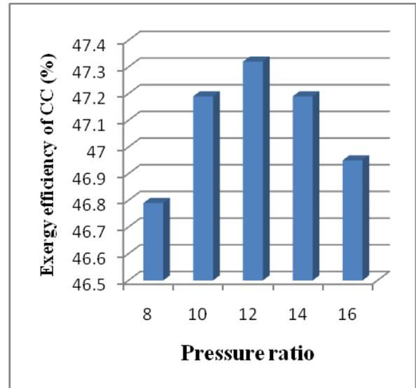
Figure 12: Effect of pressure ratio on Exergy efficiency of combined cycle.
