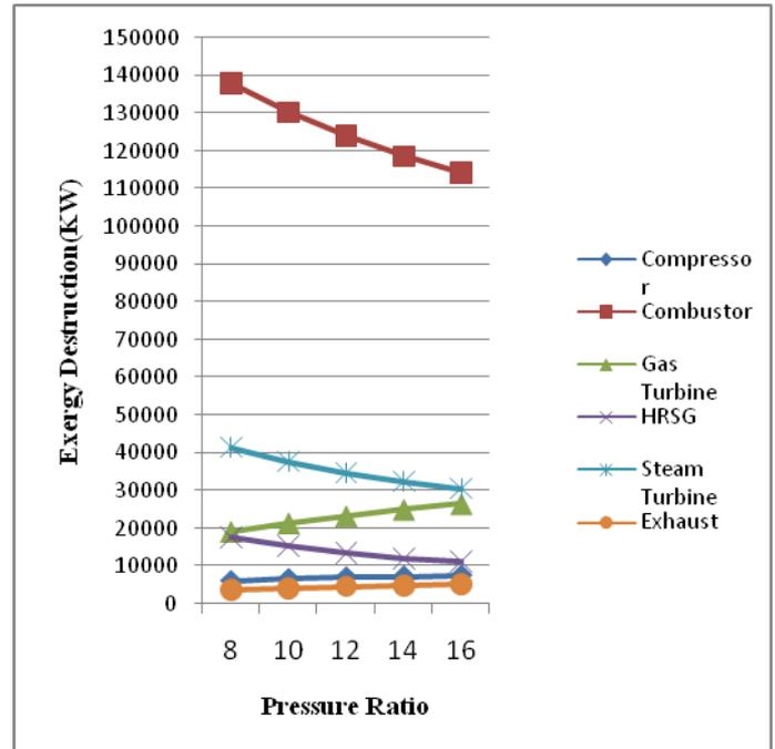
Figure 14: Effect of pressure ratio on Exergy destruction in different components of combined cycle at TIT 1100°C.
