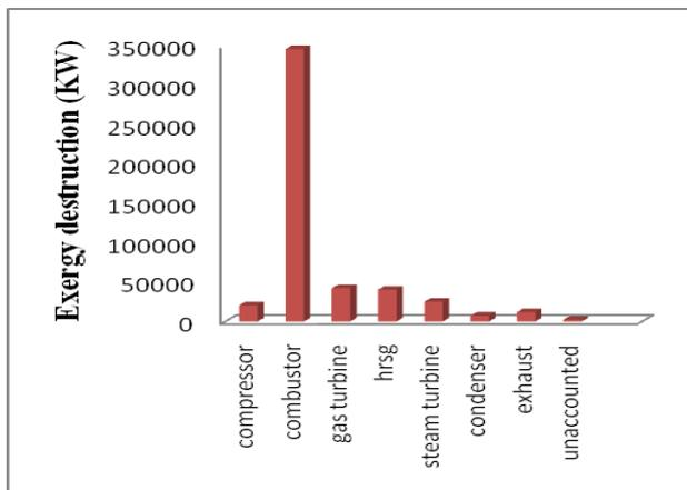
Figure 4: Exergy destruction rate at different components of the plant at TIT = 1005<sup>0</sup>C and T<sub>0</sub> =27<sup>0</sup>C and R<sub>p</sub> = 12.2.
