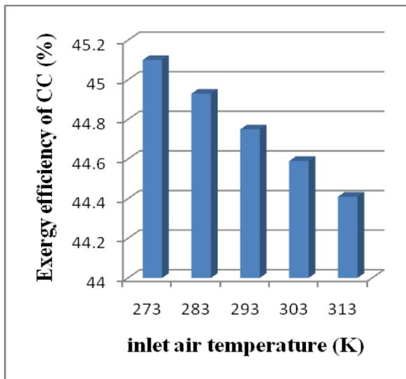
Figure 6: Effect of inlet air temperature on Exergy efficiency of CC.
