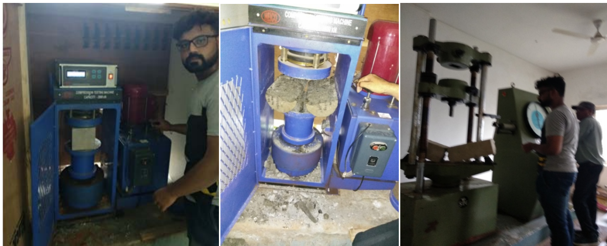
Figure 2: Compression, Split Tensile and Flexural Test Machine.
